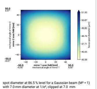
spot diameter at 86.5 % level for a Gaussian beam (M<sup>2</sup> = 1 with 7.0 mm diameter at 1/e<sup>2</sup>, clipped at 7.0 mm field size and mirror distances as given above for a two mirror scan system
