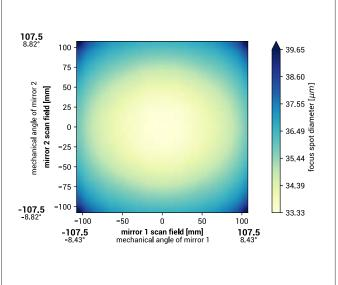
spot diameter at 86.5% level for a Gaussian beam (M² = 1) with 20.0 mm diameter at  $1/e^2$ , clipped at 20.0 mm field size and mirror distances as given above for a two mirror scan system
