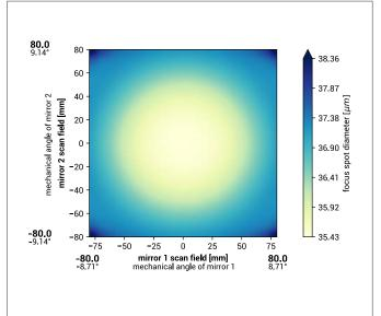
spot diameter at 86.5% level for a Gaussian beam ( $M^2$  = 1) with 14.0 mm diameter at  $1/e^2$ , clipped at 14.0 mm field size and mirror distances as given above for a two mirror scan system
